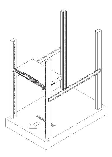
Figure 2-1. Installing the Chassis into a Rack
